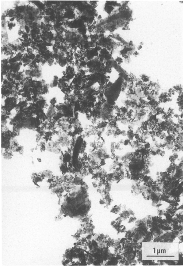
Figure 10 Transmission electron micrographs of muscovite ground for 24 h in methanol.
