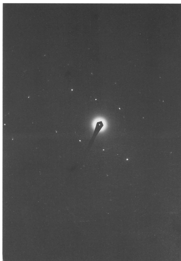
Figure 14 Transmission electron micrograph of muscovite ground for 12 h in methanol in the presence of \text{Li}^+ ions.
