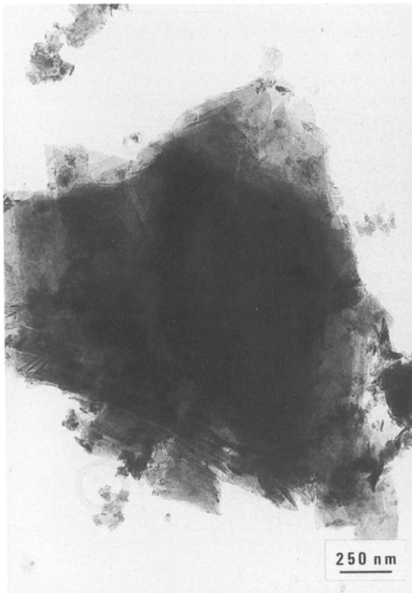
Figure 11 Transmission electron micrographs of muscovite ground for 72 h in methanol.
